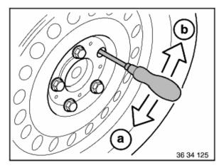
Turn adjusting screw using a screwdriver until wheel or brake disk can no longer be turned.
