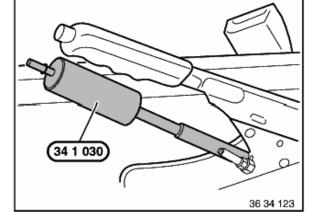
Unscrew locknut using special tool 34 1 030 and loosen cable completely.
