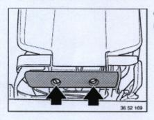
Only Coupé with mechanical seat adjustment: Remove screws and shoe guard.
