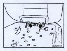
Fold up cloth tab and remove screws.
