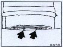
Loosen retainers on backrest shell.
