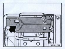
Unscrew screw and remove shoe guard at bottom.
