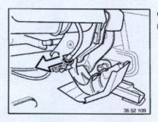
Only Coupé with mechanical seat adjustment: Pull off retainer.
