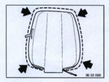
Lift out cover all around and remove together with padding (foam rubber).
