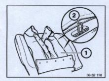
Fold cushion cover (1) together and cut off retainers (2) in padding (foam rubber). Remove cushion cover.
