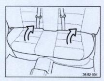
Unclip rear set cushion on left and right and lift out.
