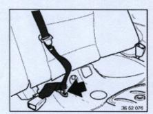
Unscrew bottom seat-belt bolt. Installation:
