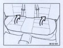
Unclip rear set cushion on left and right and lift out.
