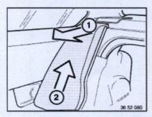
Unclip (1) the backrest side section and remove in upwards direction (2).
