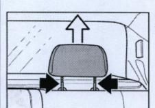
Move head restraint up as far as possible. Work gently forward and back at guides and ease up to remove.
