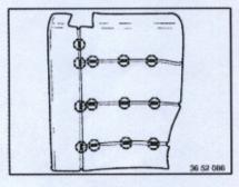
Unclip retainers and remove cover.
