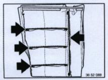
Pull securing rods out.
