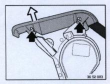
Unclip plate at left and right and remove it.
