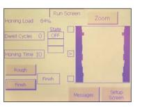
The patented SV-10 bore profile display provides a real time graphical display of the bore cross section. Photos show bore as honing cycle "starts" (top) and just before the workpiece is to "size" (bottom).
