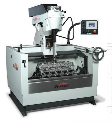
The Sunnen® SV-10 is designed with power, precision, durability and advanced technology to deliver state-of-the-art performance ... perfect for honing big, heavy or odd shaped workpieces.
