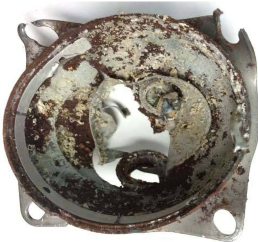
A Takata air bag inflator that deployed in 2014. The driver was killed by metal shards.
